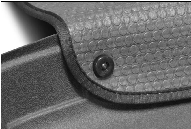
Detail of plastic knurled screw + nut.
